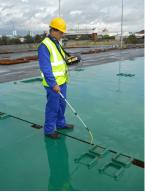
accuracy. The size of the problem can also be established from the strength of the signal detected.
