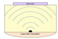
The CARGO-SAFE hatch cover leak detection system has three levels of emitters: upper, lower and vertical. This means that all the ultrasound is directed to the hatch covers, optimising its effectiveness. The diagram shows the dispersion pattern of the ultrasonic signal emanating from the CARGO-SAFE transmitter. The high sound pressure level is ample to fill the largest of holds enabling reliable and accurate readings to be taken.
